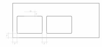
The minimum gap between a cutout and the edge of the slab must be at least 2". The size recommends distances greater than 2" when the kitchen design allows as it makes the countertop firmer.
